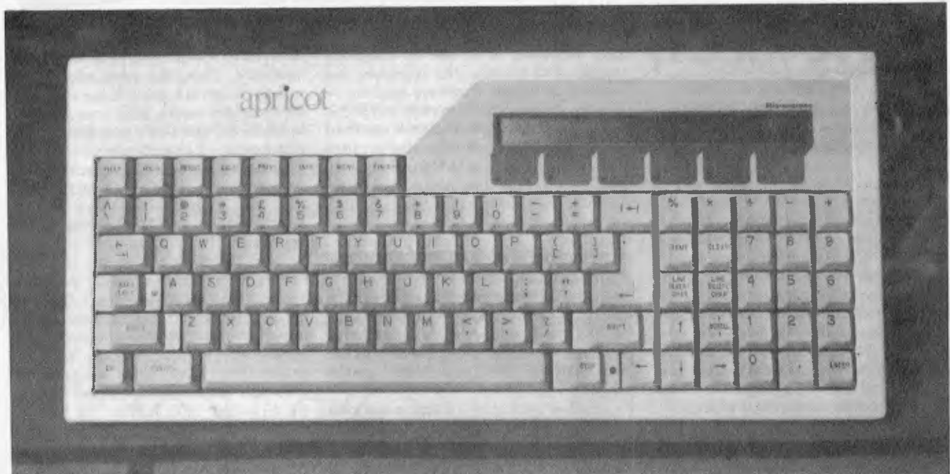
The keyboard is clearly in a class of its own with its outstanding feature being the two-line character LCD Microscreen. Being a British machine the pound sign is included and will not be removed on versions sold in Australia.
